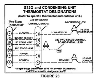
9 - Install room thermostat according to instructions provided with thermostat. See figure 28 for thermostat designations. If furnace is being used with heat pump refer to FM21 installation instruction.
